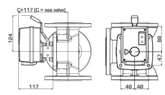
Installation dimensions for Controller Series 90K with ESBE VRG100, VRG200, VRG300 and VRB100 mixing valves
