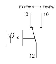
Fx: rel. humidity of the air (actual value) Fw: humidity adjusted with the wheel (set point)
