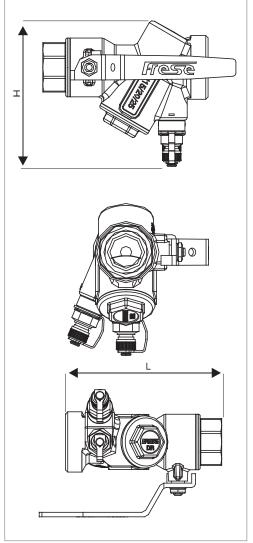
The pipe system shall be properly ventilated to avoid risk of air pockets. Glycolic mixtures up to 50% are applicable (both ethylene and propylene).
