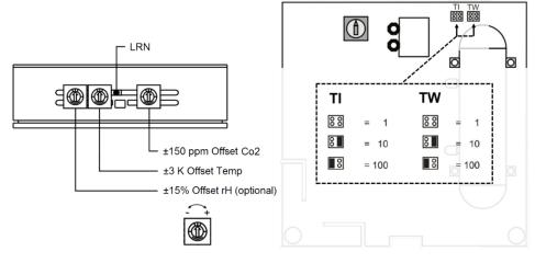
Factory default:(TW) T\_wake up = 100, (TI) T\_interval = 10Example:T\_send = 100 seconds wake up \* 10 interval = 1.000 seconds = ca. 16 minutes
