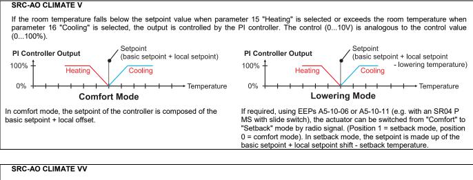
If the room temperature falls below the neutral zone, the "heating" output is activated by the PI controller. The control (0...10V) is analogous to the control value (0...100%). In normal operation, the status of the respective active output is signalled by the Prog LED (output active = LED lights up). If the room temperature exceeds the neutral zone, the "cooling" output is activated by the PI controller. If the room temperature is within the neutral zone, both output oV.
