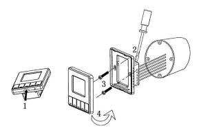
For Installing or repairing, please make sure the power is disconnected. Insert the screw driver in the plastic teeth of thermostat. Clockwise rotation of the screwdriver will separate front cover from base plate. Please follow the wiring diagram to connect the wires.
