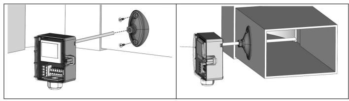
Optional mounting with mounting base (Item No. 631228), please note the installation depth of the sensorpocket. (permissible ambient temperature -35..+70  $^{\circ}$ C)
