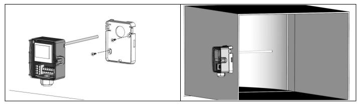
Mounting with immersion pocket or compression fitting for usage in liquid media. Use contact fluid for better heat transfer between sensor and measuring medium.
