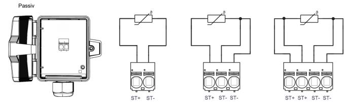
fig. (terminal assignment passive sensor)
