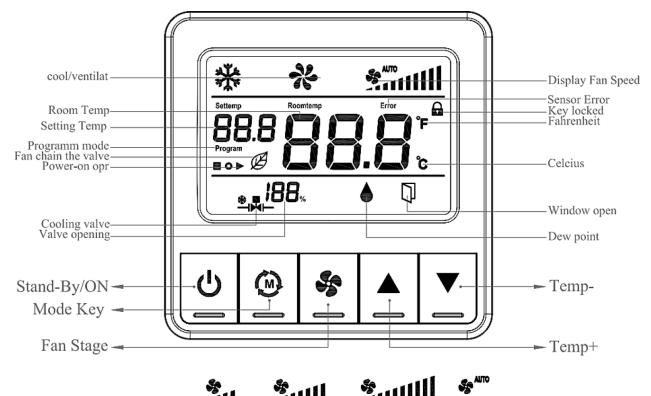
Display Fan Speed: Fan Low Fan Medium Fan High Fan Auto Page 4 / 8 Issue Date: 04.03.2022
