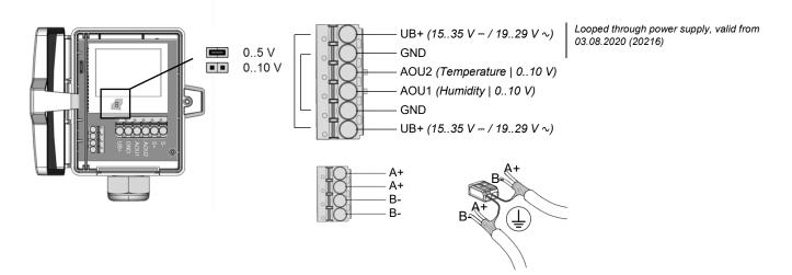
The BACnet address of the device is set binary coded in the range of 1 ... 127 via 7 dip-switches. (the address 0 is reserved and cannot be selected).
