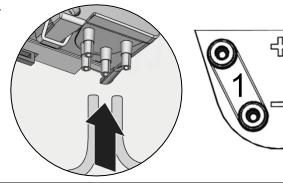
**4.** Connect pressure tubes to the duct connection pieces
