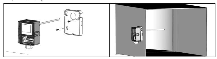
Mounting with immersion pocket or compression fitting for usage in liquid media. Use contact fluid for better heat transfer between sensor and measuring medium.
