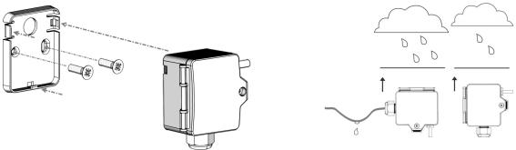
Regardless of the compass direction, the outdoor sensor should not be mounted in the following locations:
