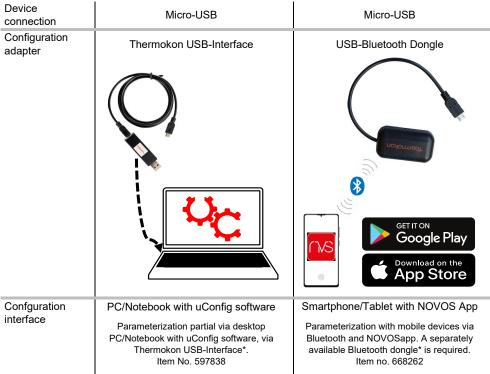
\*Commercially available Bluetooth dongles or USB to Micro-USB adapter cables are not compatible. You need a mobile device that supports at least Bluetooth version 4.1. The configuration app with the corresponding instructions can be downloaded from the Google Play Store or the Apple App Store.
