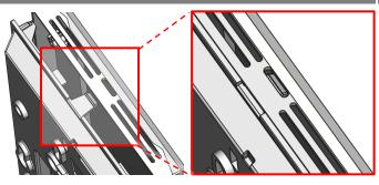
Fix the upper part of the housing on the underside with the screw
