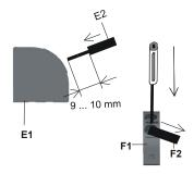
figure 11: Connecting/disconnecting mains and load circuit
