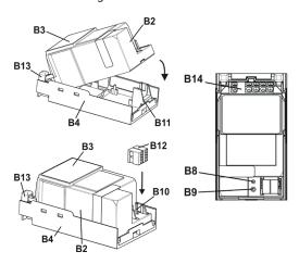
figure 7: mounting of an RL module
