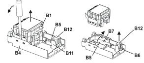
figure 6: dismounting an RS module
