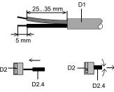
figure 10: Connecting / Disconnecting bus cables
