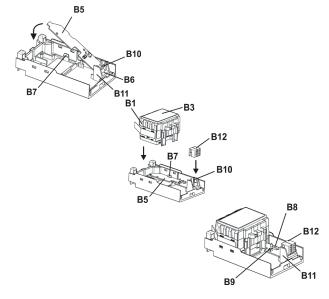
figure 5: mounting of a RS module
