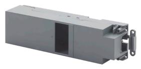
The AP 118 Control Module Box with a height of 41 mm is designed for installation in a false ceiling, in a raised floor, directly on a wall or in an installation channel or raceway. The Control Module Box is affixed with screws at the two ends of the housing.
