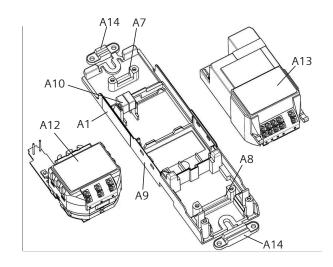
figure 4: mounting / dismounting of RS/RL modules
