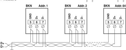
The wiring of the line for BACnet (MS/TP) / Modbus (RTU) is to be carried out in accordance with applicable RS485 regulations.
