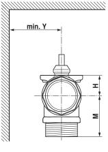
X/Y: Minimum distance with respect to the valve centre. The actuator dimensions can be found on the respective actuator data sheet.
