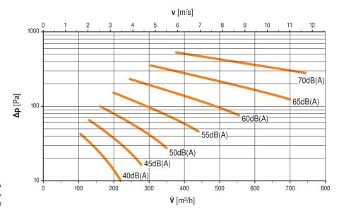
$\begin{array}{c} \text{Volumetric flow } \dot{\text{V}} \\ \text{Air velocity v} \\ \text{Pressure loss } \Delta \text{p} \end{array}$
