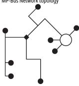
There are no restrictions for the network topology (star, ring, tree or mixed forms are permitted). Supply and communication in one and the same 3-wire cable
