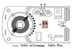
Factory setting Switch **a** at 10° Switch **b** at 80°
