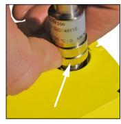
For mounting the probe must be plugged into the socket and screwed on the sensor by turning the lower knurled screw clockwise. Tighten hand-screwed only.
