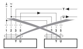
Control with 4...20 mA via external resistor
