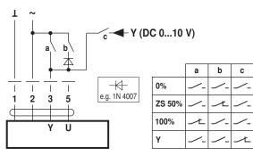
Override control with AC 24 V with rotary switch
