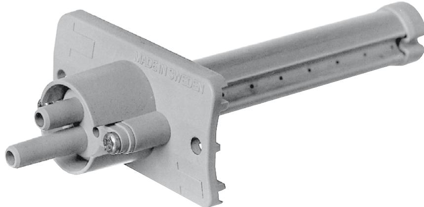
The GV sensor is intended for direct in-duct installation primarily in VAV boxes. It measures the air velocity across the cross-section of the duct. An output signal is then transferred to the measurement chamber in the VAV controllers TAC 224V and TAC 224VL.
