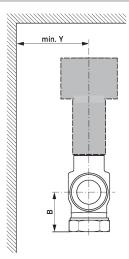
X/Y: Minimum distance with respect to the valve centre.
