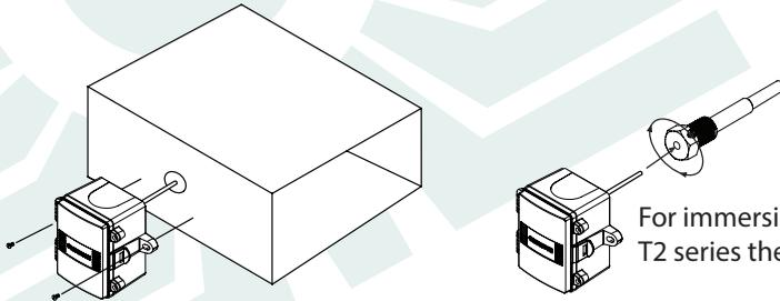
For immersion applications, T2 series thermowell is required.
