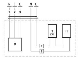
M = Actuator T (°C) = Thermostat H = Heating
