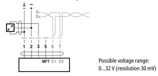
Modbus RTU / BACnet MS/TP with analogue setpoint (hybrid mode)
