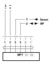
Requirements for switching contact: The switching contact must be able to accurately switch a current of 16 mA @ 24 V.
