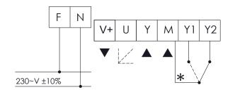
\* Floting only sink (connect Y1, Y2 to M)
