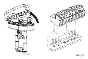
**Note**: To avoid damages to electronic components caused by the PCB bending, do not press too much while fixing the terminal block
