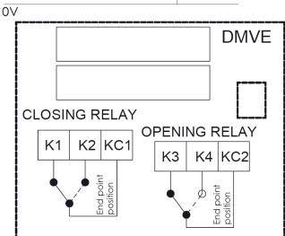
(\*) MVE contain a half-wave rectifier power supply. They must not be powered with transformers that are used to power other devices using not isolated full-wave rectifier power supply.
