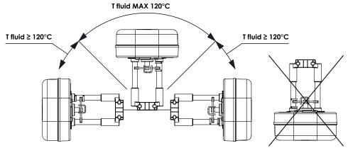
To mount the actuator on to a valve, position the valve stem to the bottom of its travel, slide the actuator onto the valve neck, adju-
