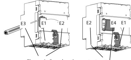
Figure 4: Covering the contact system
