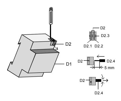
Figure 3: Attaching / removing the bus terminal
