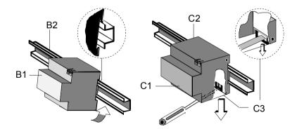
Figure 2: Installing / dismantling the device
