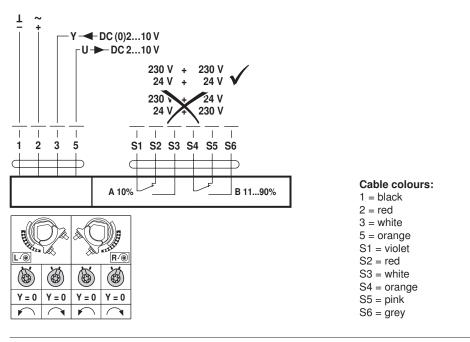
Rotary actuator fail-safe, modulating, AC/DC 24 V, 10 Nm, with 2 integrated auxiliary switches
