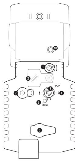
1 Direction of stroke switch Switch over: Direction of stroke changes Cover, POP button 2 POP button 3 Scale for manual adjustment 4
