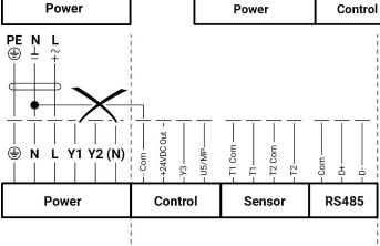
Power supply must not be connected to the signal terminals!
