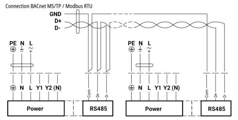
Connection BACnet MS/TP / Modbus RTU with analog setpoint (hybrid mode)
