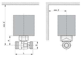
X/Y: Minimum distance with respect to the valve centre. The actuator dimensions can be found on the respective actuator data sheet.
