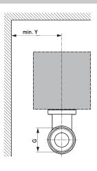
$\ensuremath{\mathsf{X/Y:}}$  Minimum distance with respect to the valve centre.
