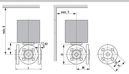
X/Y: Minimum distance with respect to the valve centre. The actuator dimensions can be found on the respective actuator data sheet.
