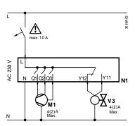
N1 RDF310.2/MM V3 3-wire on/off (SPDT) zone valve M1 3-speed fan
