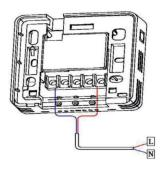
Step 2: Connect the wires the same as the picture. The detailed connect way refer to the wiring diagram.
