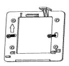
Step 1: Take out the screws and board from the box, then fix the board on the wall the same as the pictures.
