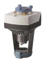
Electromotive actuator to operate Siemens 2-port and 3-port valves, types VVF42..K, VVF42..KC und VXF42.. with 20/40 mm stroke, as control and safety shutoff valves on heating, ventilation, and air conditioning plants.
