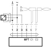
Connection with switching contact, e.g. Δp monitor
