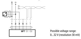
Modbus RTU / BACnet MS/TP with analogue setpoint (hybrid mode)
