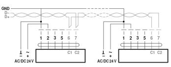
Connection with passive sensor, e.g. Pt1000, Ni1000, NTC
