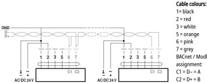
Connection with passive sensor, e.g. Pt1000, Ni1000, NTC
