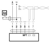
Requirements for switching contact: The switching contact must be able to accurately switch a current of 16 mA @ 24 V.
