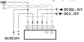
5 = orange BACnet / Modbus signal assignment: C1 = D- = A C2 = D+ = B
