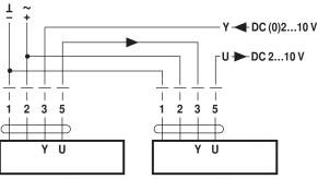
Control with 4...20 mA via external resistor
