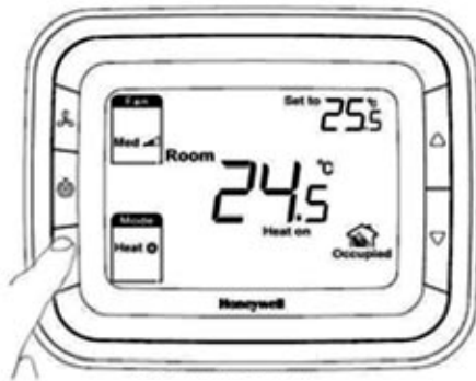
PRESS THE MODE BUTTON TO SELECT HEAT, COOL, AUTO OR VENT
