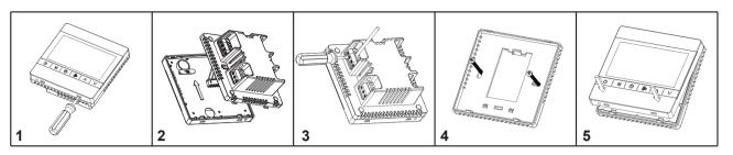
\* Remove the insulating strip before installation
