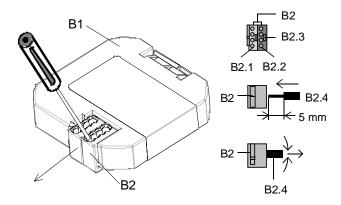
Figure 2: Connecting/disconnecting the bus cable
